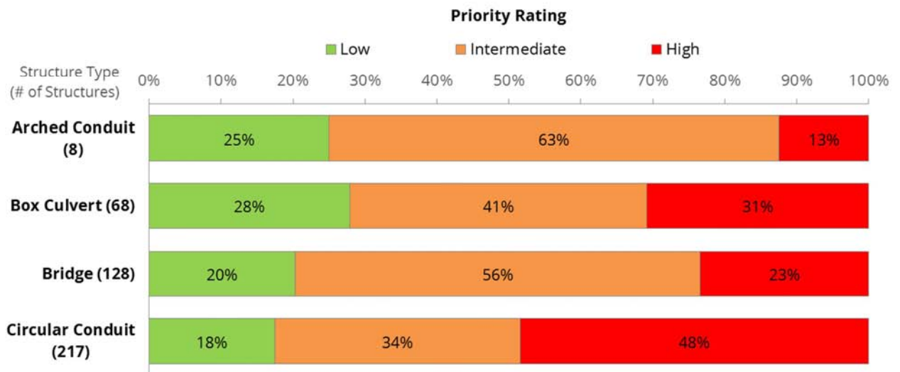
Figure 2-23. Culvert and bridge priority ratings by structure type.
